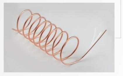
VANSAN PE2-PA winding wire consist of a solid copper conductor insulated with Polyethylene (PE2) and Polyamid (PA). PE2 sheath provides good electrical protection and a Polyamid (PA) sheath provides good mechanical.
