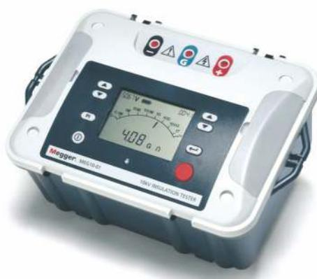
Under the normal operating conditions, a motor inside the well should have 2 megaohm insulation resistance. When the insulation resistance drops under 0.5 megaohm, there might be an insulation problem in winding. Test voltage should be at least 500 V DC.
