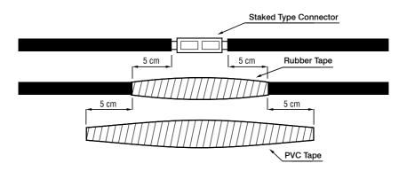
Total thickness of tape should be no less than the thickness of the cable insulation in order to prevent the smashing of the cables when the pump is lowered in the well.
